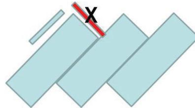
Tailpiece: must not be at an angle as shown in above picture
